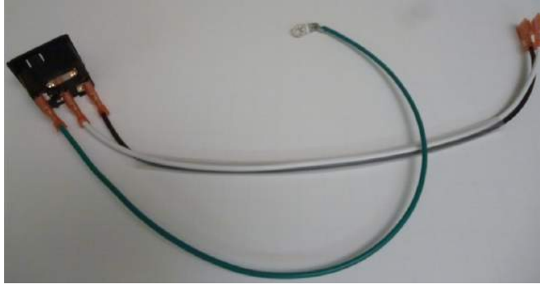
Figure 30-Wiring IEC power connector
