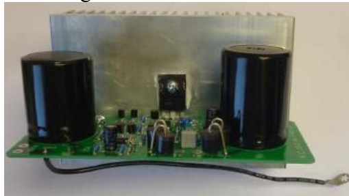
Figure 23—power supply with attached ground wire
