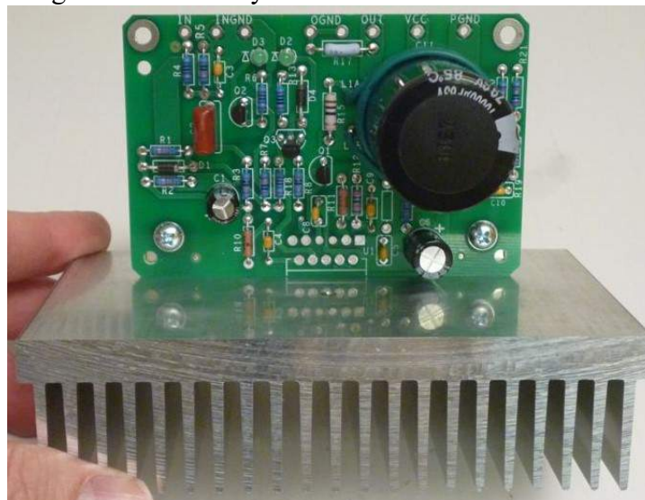
Figure 19-mounting the PCB to the heat sink
