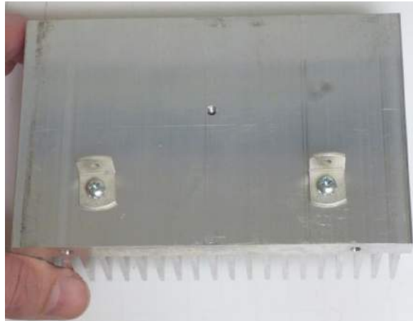
Figure 6-Note the rounded brackets used for the power supply heatsink and PCB
