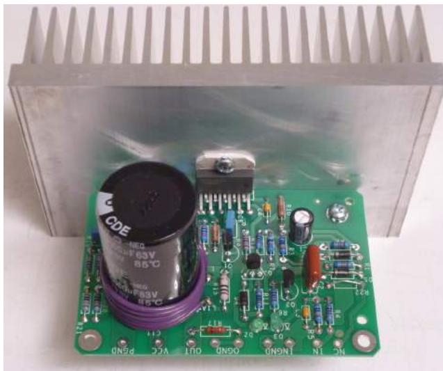
Figure 20-a completed amplifier module
