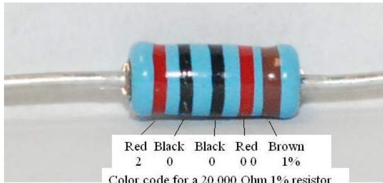
Figure 46-demonstrating the resistor color code
