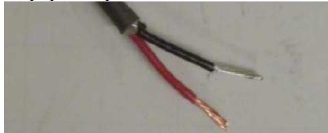
Figure 47- Shield wire end prep completed
