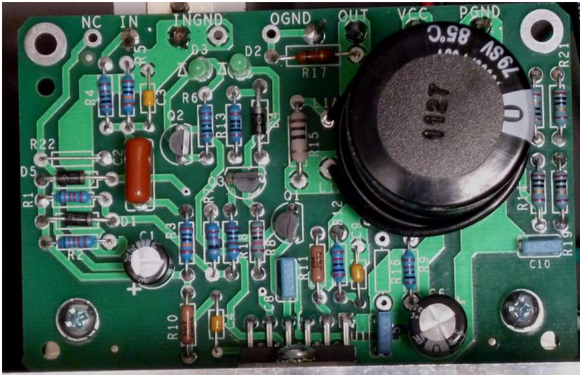
Figure 12-Closeup of Completed Amplifier board
