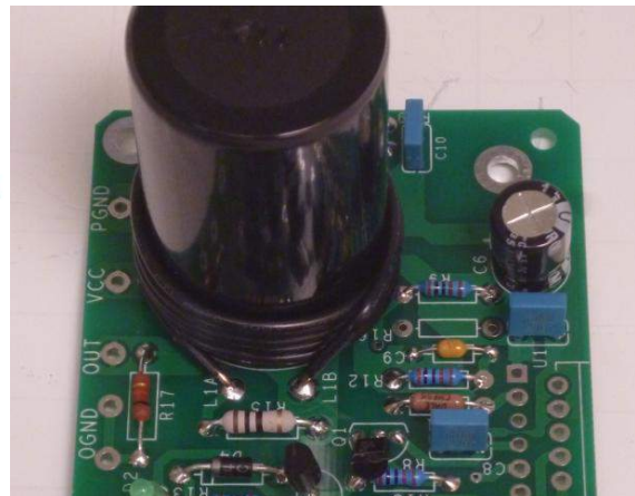
Figure 17-finishing step for the output inductor
