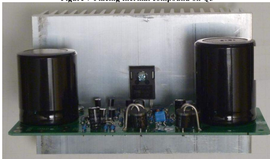
Figure 8-Installing Q5 on the heatsink and to the PCB
