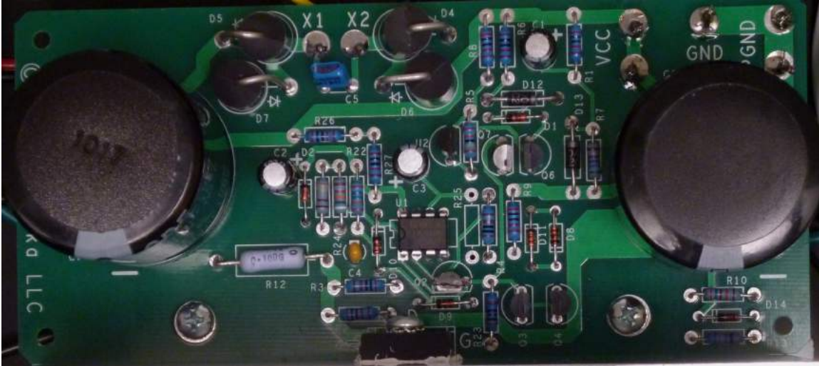
Figure 10-Assembled Power supply mounted on heat sink
