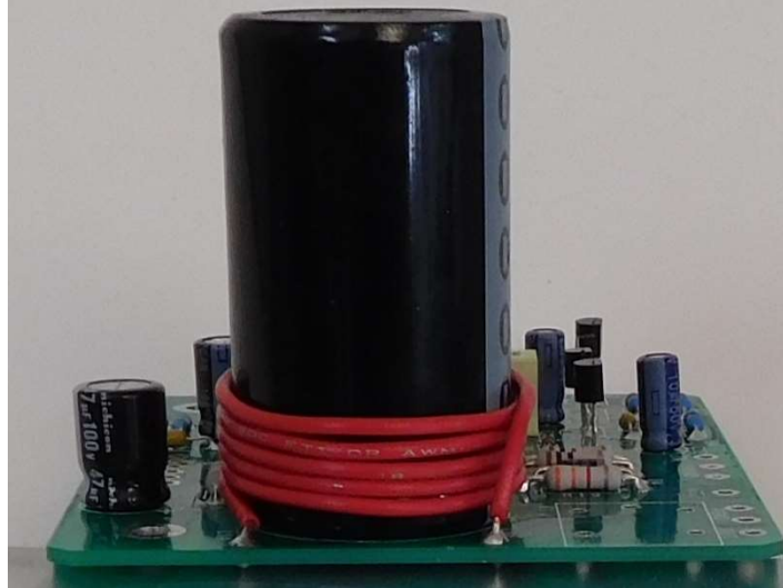
Figure 16-finished step for the output inductor
