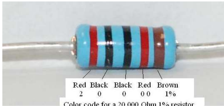
Figure 46-demonstrating the resistor color code
