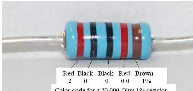
Figure 46-demonstrating the resistor color code
