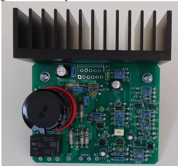
Figure 18-mounting the PCB to the heat sink
