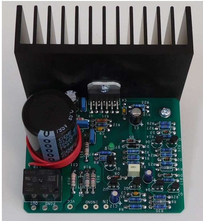
Figure 20-a completed amplifier module
