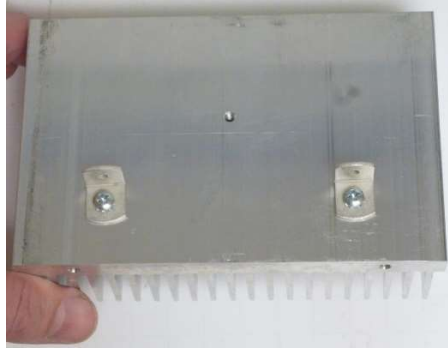
Figure 5-Note the rounded brackets used for the power supply heatsink and PCB
