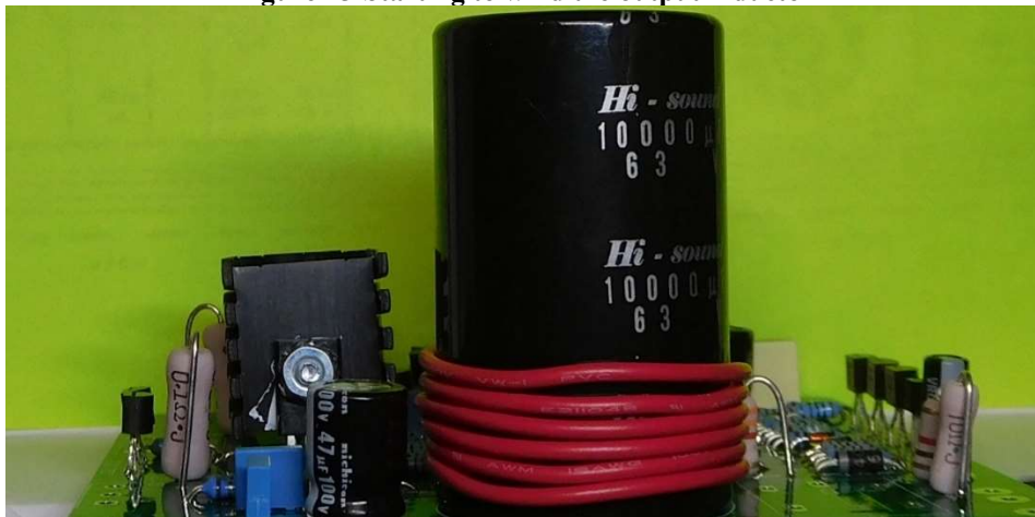
Figure 16-finishing step for the output inductor
