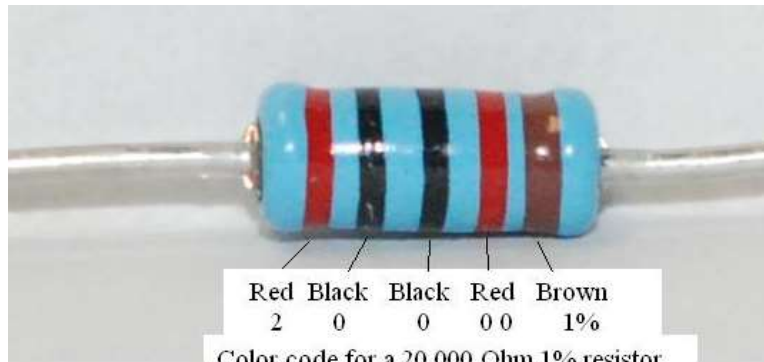
Figure 54-demonstrating the resistor color code
