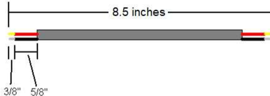
Figure 31-shielded cable for left channel. Right channel has overall length of 11 inches.
