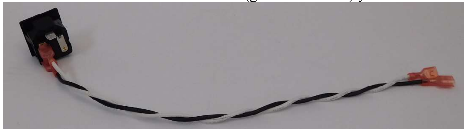
Figure 37-Wiring IEC power connector line and neutral
