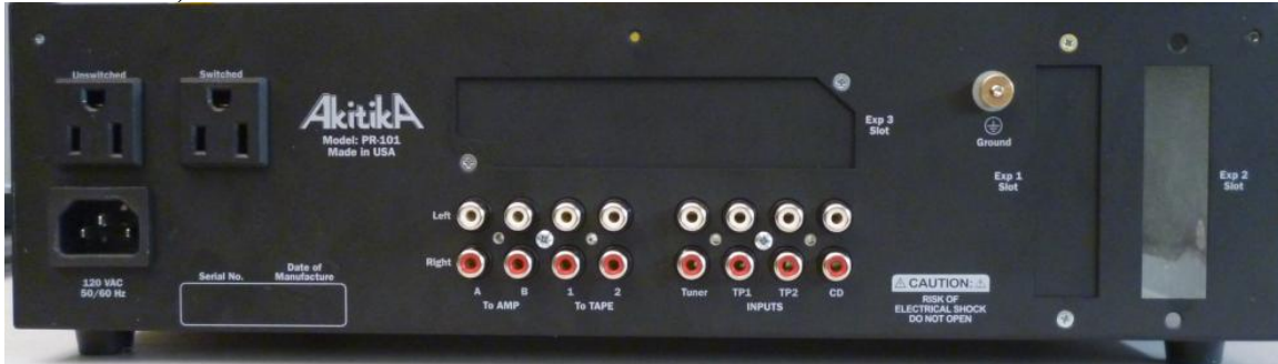
Figure 47-Two of the three cover plates have been installed
