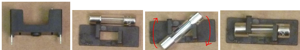
Figure 3-Fuse holder body solders into board, installing fuse into lid of fuse holder
