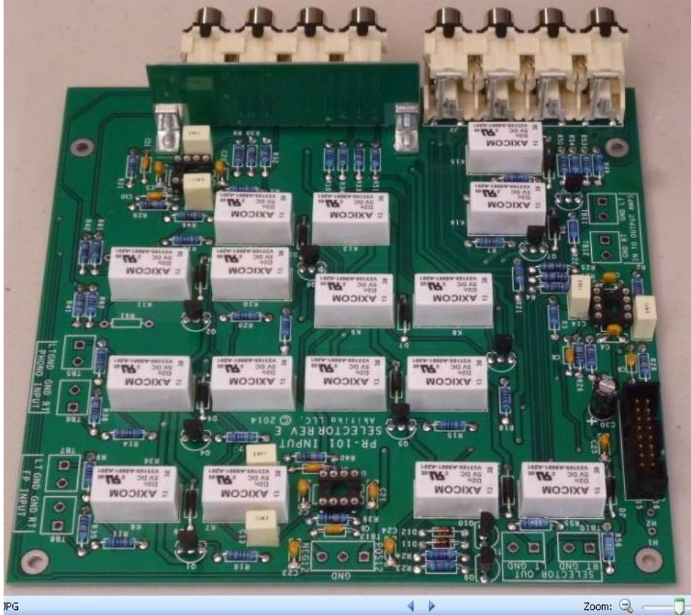
Figure 34-Assembled Input Selector board (some kits have black relays)
