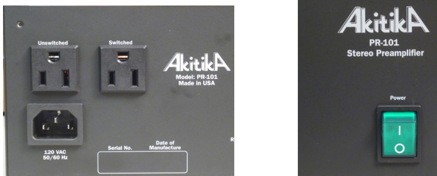
Figure 13-Installing power outlets and IEC connector...watch orientation! Installing the power switch...watch orientation!
