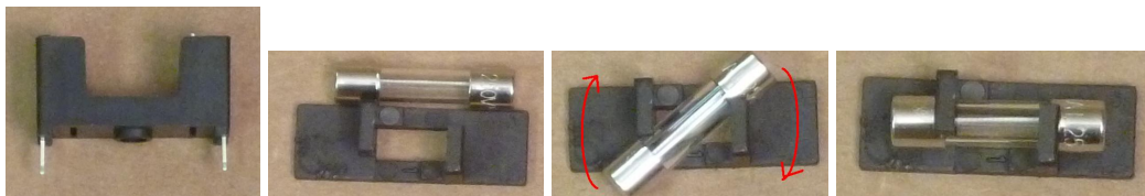
Figure 3-Fuse holder body solders into board, installing fuse into lid of fuse holder
