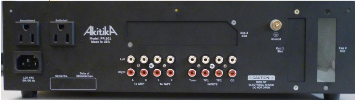
Figure 50-Two of the three cover plates have been installed
