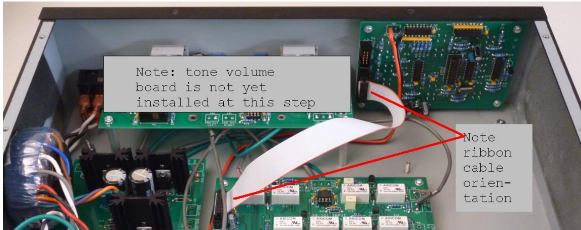
Figure 36-16 pin ribbon cable orientation and installation
