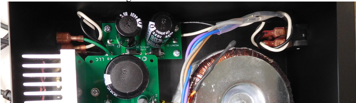
Figure 4-DC scraper installed into a GT-102
