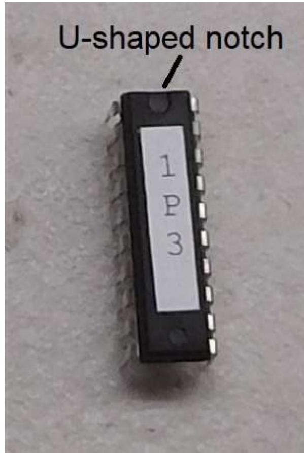
Figure 1-Remember that the U-Shaped Notch goes toward the bottom of the socket
