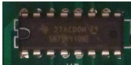
Figure 31-Remember to match silk screen and IC orientation mark
