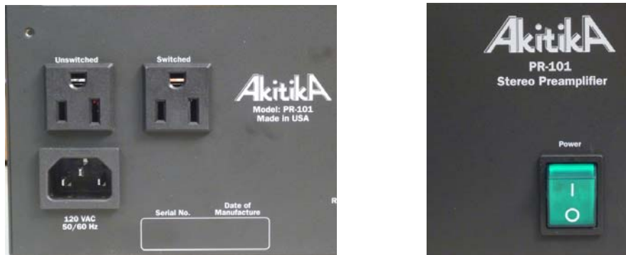
Figure 12-Installing power outlets and IEC connector...watch orientation! Installing the power switch...watch orientation!
