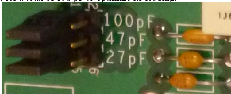
Figure 9-No additional capacitive loading is selected with the short plugs as shown here
