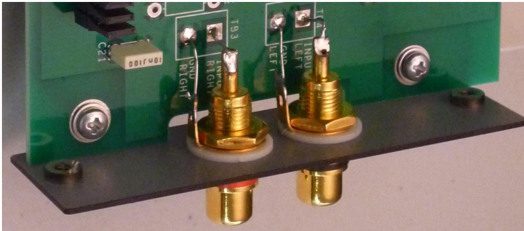
Figure 7-Install both jacks, noting orientation of ground lugs, color stripes, and solder terminal
